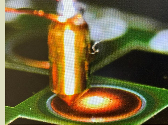
Spring Pin in Via Pad
