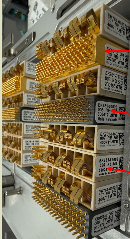
Spring pins in ATE test head interface
