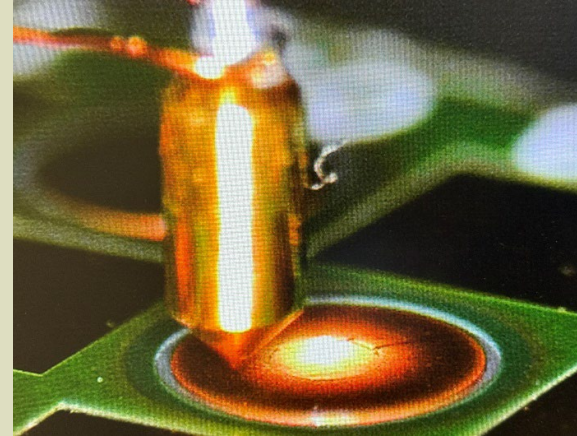
Spring Pin in Via Pad
