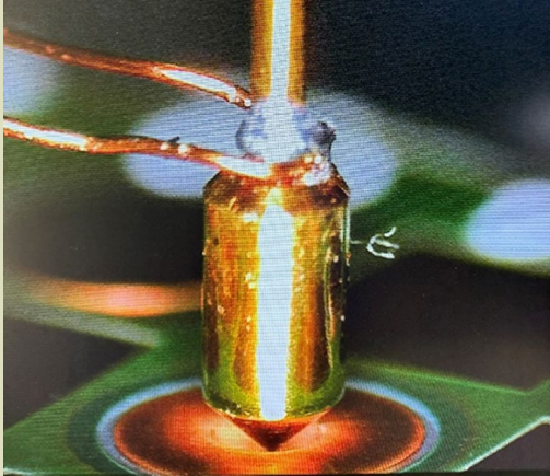
Spring Pin in Via Hole
