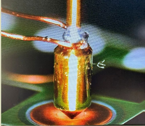
Spring Pin in Via Hole
