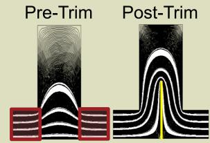
Trim is achieved by making a series of overlapping laser blasts in a resistor to divert current flow into a longer path, increasing the effective resistance
