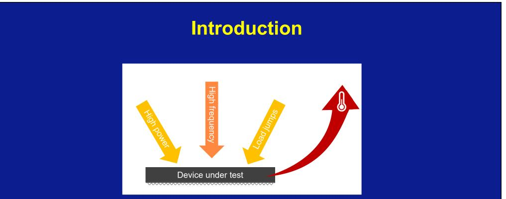
**Thermal influences** on an IC device under test due to new chip technologies makes it more and more difficult to keep the test temperature near the set point.
