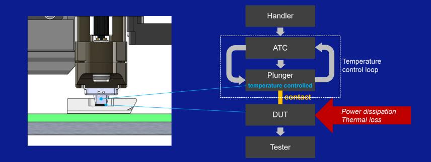
ATC controls the contact plunger temp. without recognizing / reacting to external influences on the device immediately.
