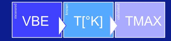
$T_{max}$  can vary between different devices > PDC can recalculate  $T_{max}$  based on the **T** and **V**<sub>BE</sub> for each device individually.
