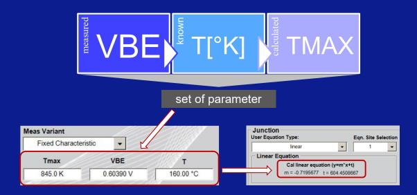
$V_{BE}$  (measured) at T (known) →  $T_{max}$  (calculated) > gain & offset of linear function →  $T_{junction}$  (calculated by PDC)
