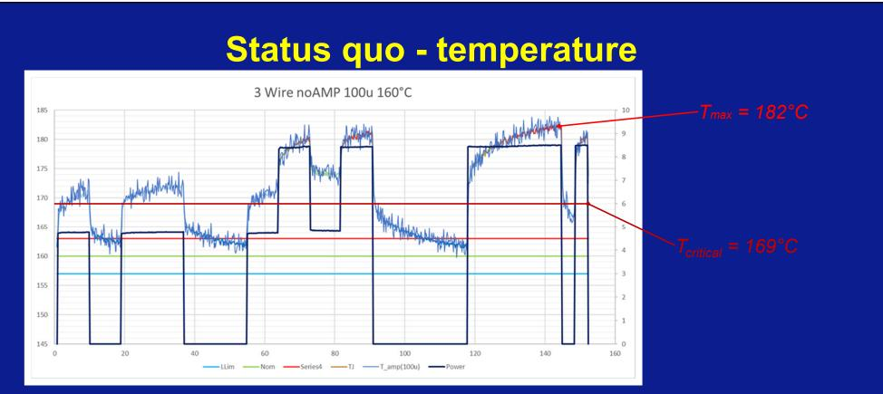
This graph shows a real case study. As a result of the power dissipation, the device temperature rises rapidly by more than **20K** when **8W** power is applied.
