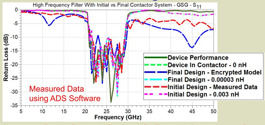
Putting Device in Contactor for Test adds Inductance to System
