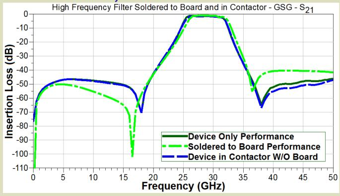
Load Board Grounding has Effects on Filter Out-of-Band Rejection
