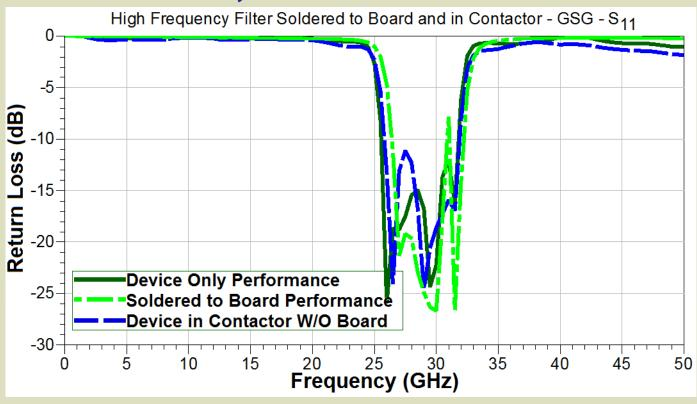
Load Board Grounding has Effects on Filter In-Band Return Loss
