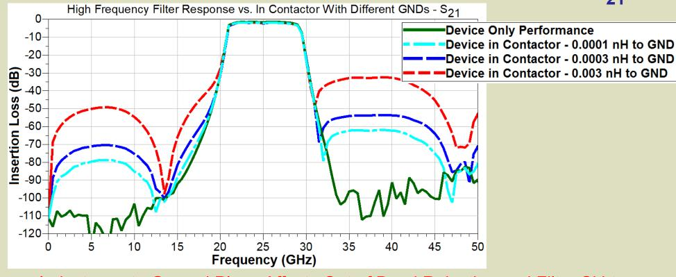
Inductance to Ground Plane Affects Out of Band Rejection and Filter Skirt
