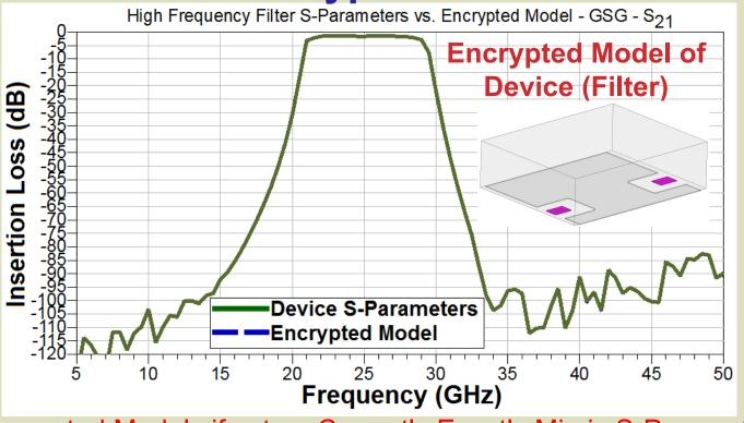
Encrypted Models if set up Correctly Exactly Mimic S-Parameter Data
