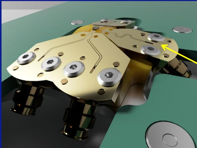
Rf signals are routed away from probe using a coplanar waveguide trace
