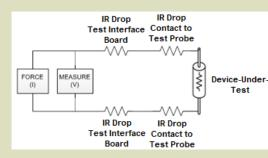
• Four wire contacting is the most accurate method when measuring resistance below 1.0  $\Omega$ .
