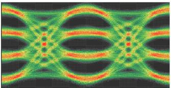
PCIeG5 @ 32 Gbps (NRZ @ 32 Gbps) is tested at BER = 10<sup>-12</sup> Typical eye mask limits are:
