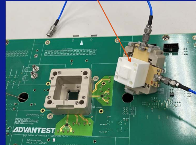
Radiating near-field OTA setup
