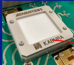
Custom socket lid made with electromagnetic transparent material
