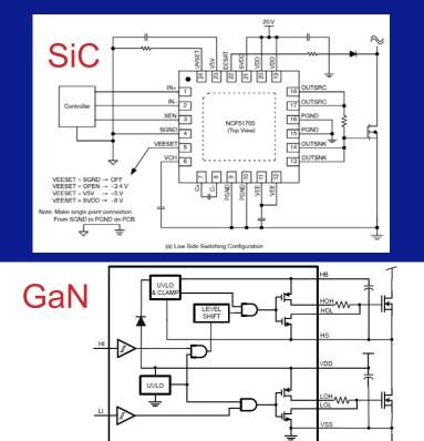
Figure 1: Optimized to drive both high- and low-side eGaN FETs, TI's driver LM5113 offers separate sink and source outputs.
