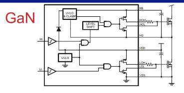
Figure 1: Optimized to drive both high- and low-side eGaN FETs, TI's driver LM5113 offers separate sink and source outputs.
