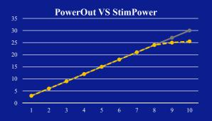
This slope works well when PA device is in "Linear Area". However if the Power Out is close to "Non-Linear Area"(NLA), this formula doesn't work.
