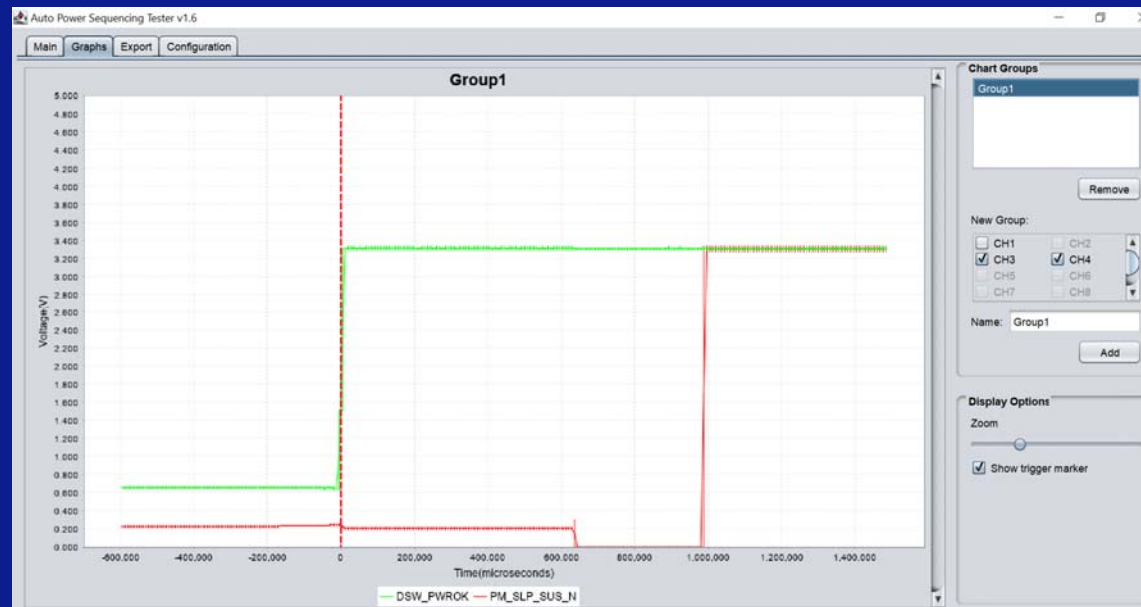
Screenshots of actual Power Sequencing Tests "Graph" Tab
