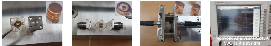
Fig. Coaxial socket measurement setup with v-type 1.85mm connector
