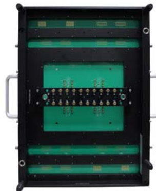
Receiver/Load Board Assembly
