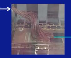
Shielded Coaxial Cables connected to shielded ceramic DUT board with traces to DUT Sockets for measurements downto pico-Ampere levels
