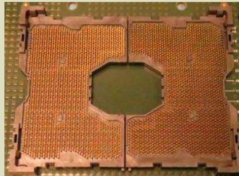
Socket is surface mounted (soldered) to board
