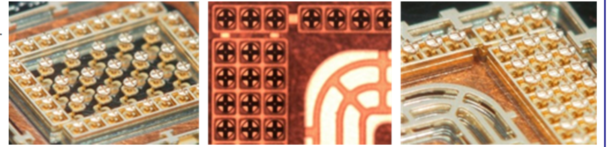
Fig. Co-axial BGA socket with rectangular ground shape
