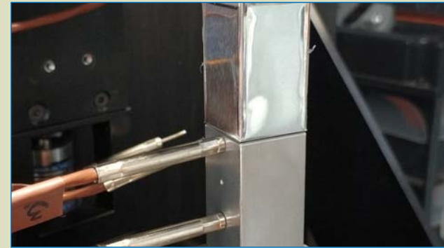
Inserting RTDs prior to Phase I start.
