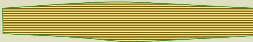
PCB Crown with standard manufacturing process
