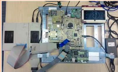
Open Chassis/ Validation Platform
