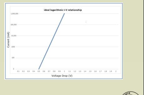
Current Measurement Using Non-Linear Passive Device
