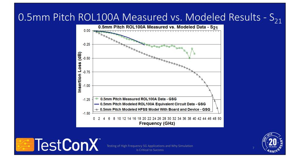
QAM and Get It! - High Frequency (HF), 5G, and millimeter-wave (mm-wave)
