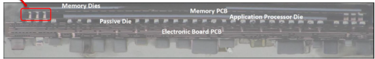
Apple A10 (iPhone 7) in TSMC InFO PoP (chips first fan-out with ECD Cu posts)
