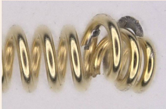
Cracked and mangled
