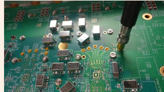
Application of board connectors and interfaces for segmented DUT signal path
