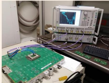
**Load Board and Test Socket**
