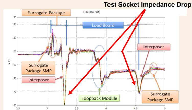
Unless measured or tested there is no assurance that a test socket for high speed SerDes I/O test impedance is ~100 Ohms differential or ~50 Ohms for single ended application.
