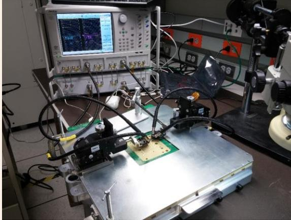
~ 50Ghz Probe setup up differential and single ended
