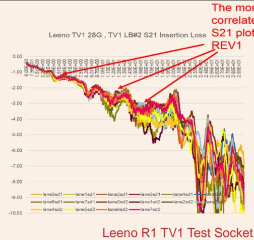
The more inductive pins correlate with rippling on S21 plots for Leeno TV1 REV1
