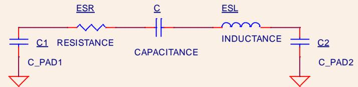
R28G Resistor equivalent circuit
