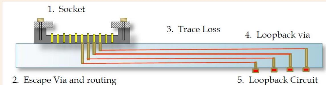
$$\text{Total Loss} = (\text{socket} \times 2) + (\text{escape}) + (\text{trace loss}) + (\text{LB via} \times 2) + (\text{LB circuit})$$
