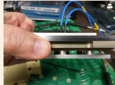
**Isolated Test Socket**
