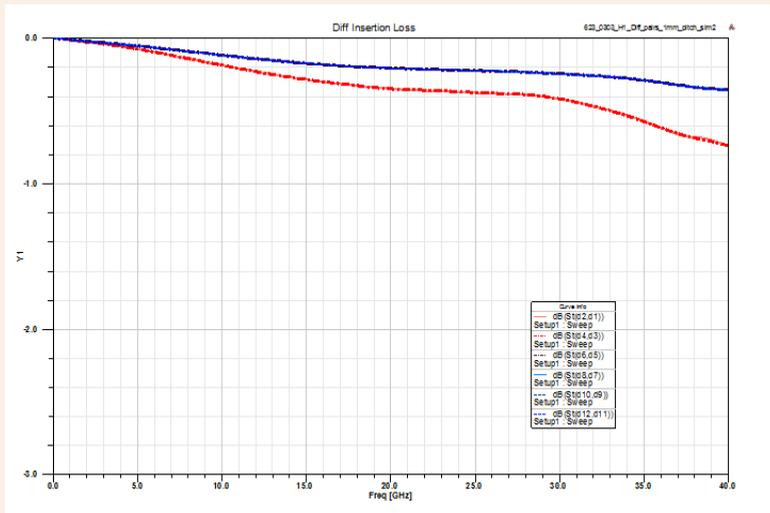
Test Socket S21 Insertion Loss
