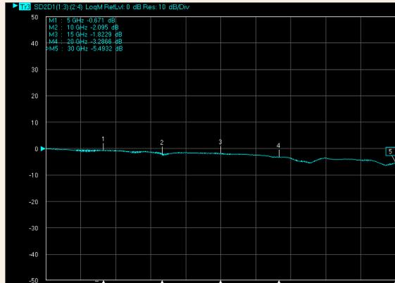
TV1 Surrogate S21 Insertion Loss Profile, TX & RX Loop
