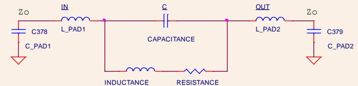
C28G Capacitor equivalent circuit
