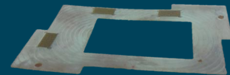
Top interposer-to-package socket: Elastomer guide (in white) Shin Etsu Interconnect (in brown)
