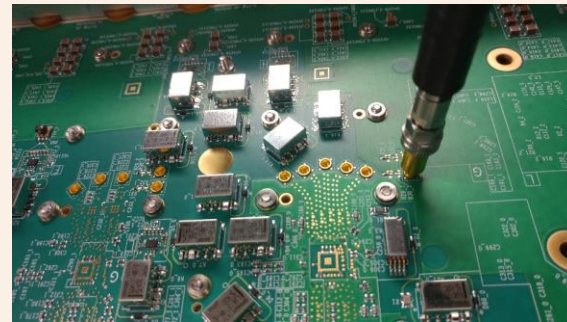
Measuring loadboard performance with SMP connectors
