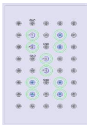
Fig 1 : Stagger differential transmission channel matrix example
