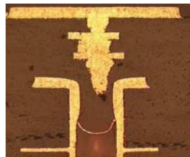
Fig 5: Stacked \mu Via over buried failure
