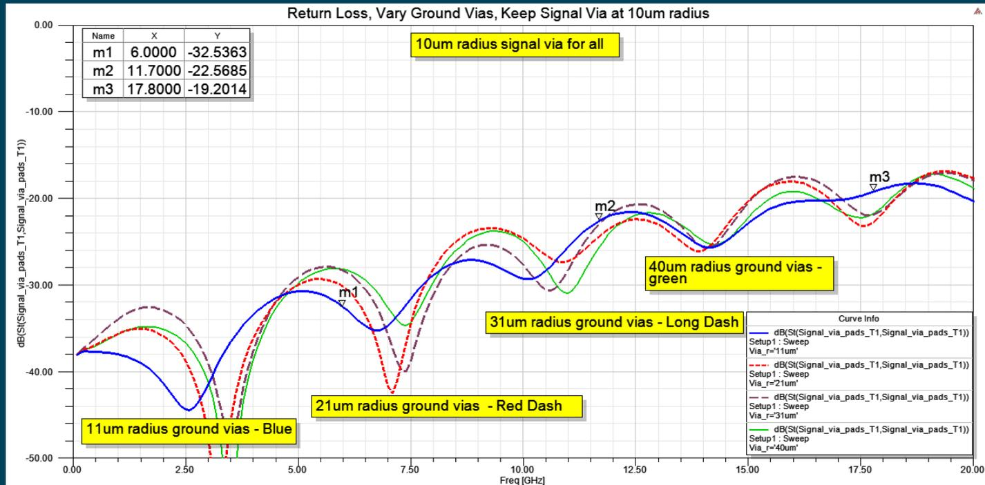
Choose Signal Via Dia. 20um & Gnd Vias Dia. 80um for higher Freq. Sweep
