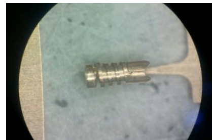
Fully assembled pin attached to the reel
