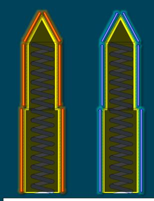
In a spring pin, the HF energy flows entirely in the outer shell completely avoiding the spring
