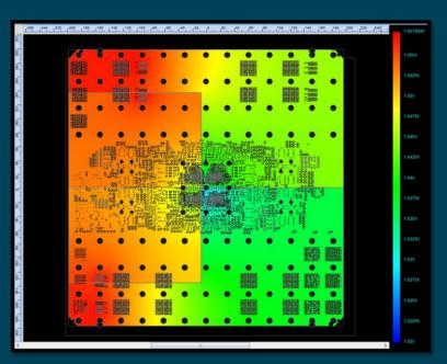
Simulation takes into account all aspects of the board design, including capacitor models, power planes routing, and socket performance
