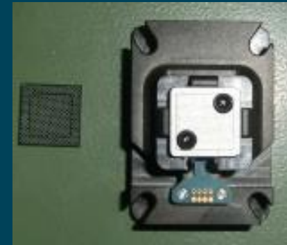
ATC Sensor routed via leadbacker to the socket
