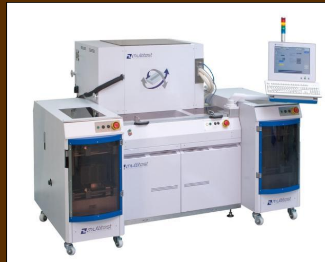
Example: Standard Strip Test Handler with MEMS Box
