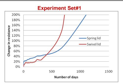
Without coating, both (swivel & spring lid) design failed around 500 days
