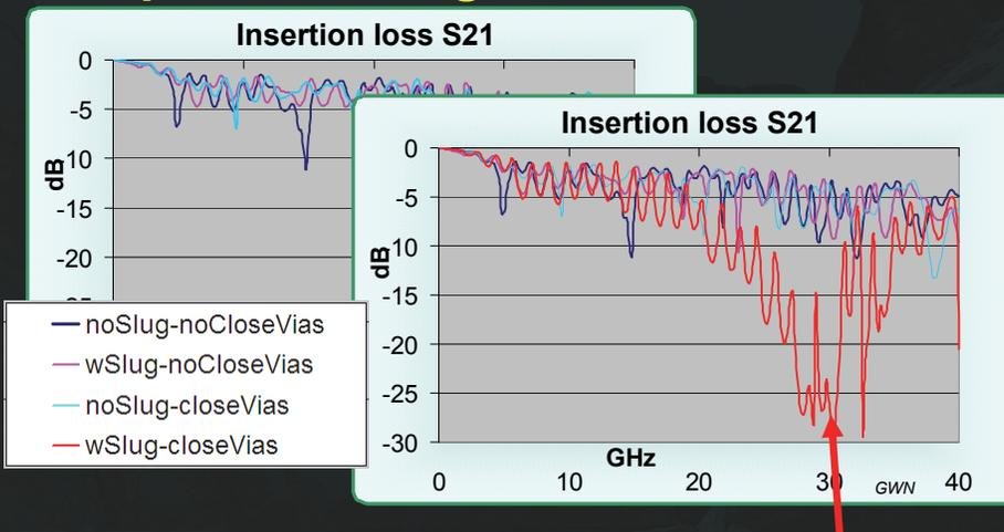
**In this case the change negatively impacts insertion loss high frequency performance if a slug is present**
