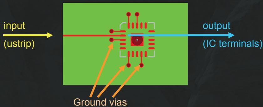
Example uses actual QFN style socket on PCB
