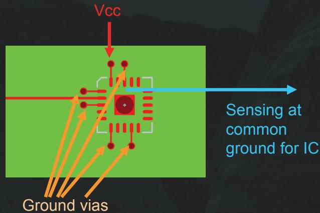
A power plane is assumed right under the ustrip ground plane in the PCB
