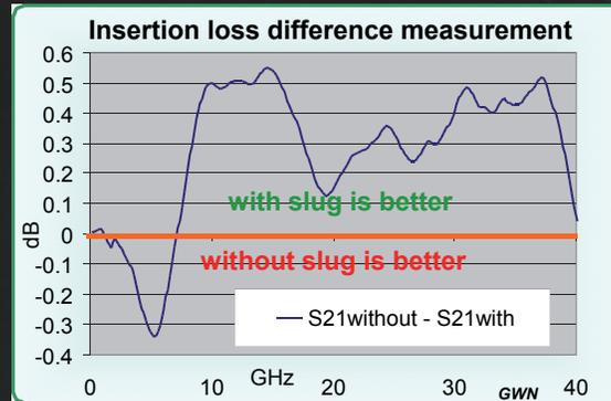
Measured on a QFN style socket (without PCB)
