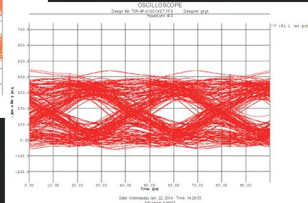
Eye diagram shows how a 28 GB/s PRBS is affected by the insertion loss drop
