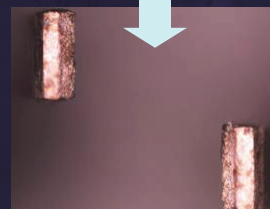
12gf New Plating @ 200 Deg. C
