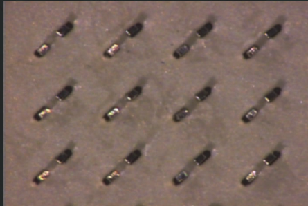
Close-up of probes in the populated area of the "universal" contactor
