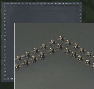
Top view of Overmolded bottom package
