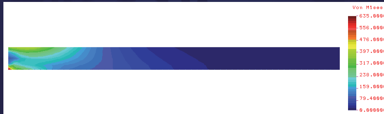
Stress contours in Silicon die using probe pin displacements (in MPa)
