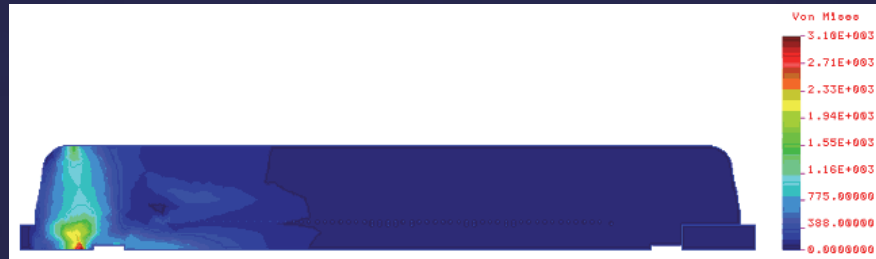
Stress contours in package using probe pin displacements (in MPa)
