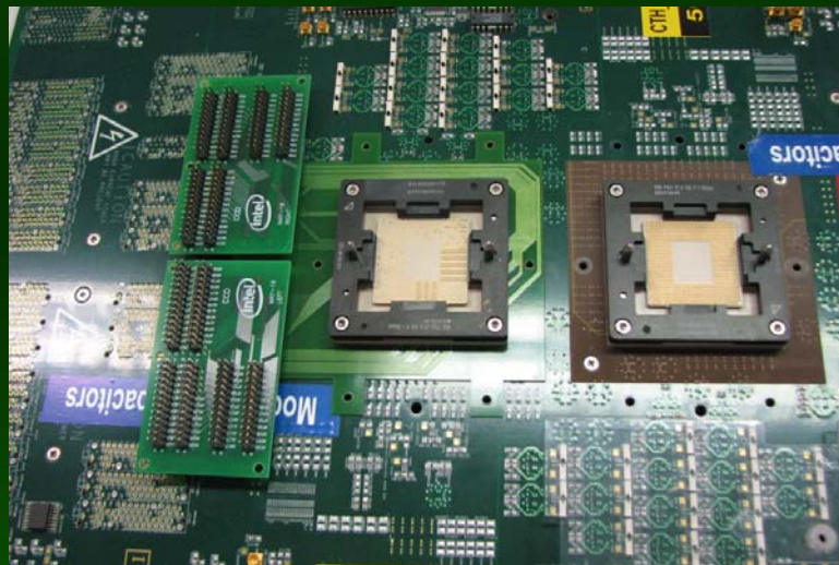
Pin Grid Array Current Sense Interposer Application Featuring Vertical Embedded Resistors
