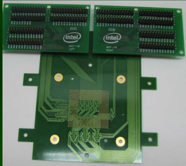
Pin Grid Array Current Sense Interposer Application Featuring Vertical Embedded Resistors
