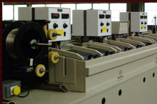
A typical continuous wire plating line.
