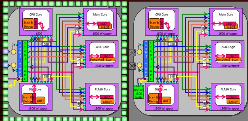
There are 2 physical Vias – each die has its own TAP that operates simultaneously and those TAPs are addressed by 1149.7 2-wire interface
