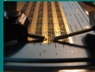
Testbed for an array of micro-contactors (wafer probing, 150 \mu m pitch)
