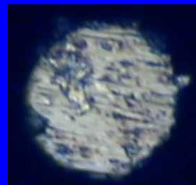
Probe tip after only 5 TD's on a “clean” pad.
