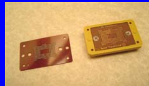
Socket Assembly with Space Transformer
