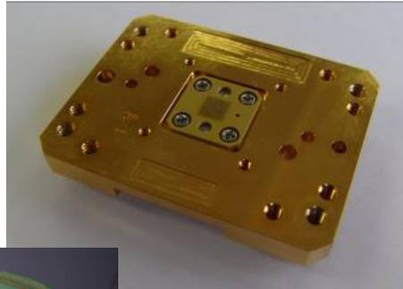
0.3mm pitch WLCSP Test Socket
