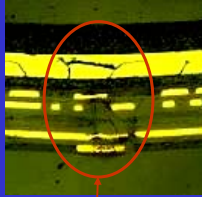
Cracks on die, substrate and molding
