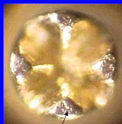
Solder Contamination & Flattened Crown Points
