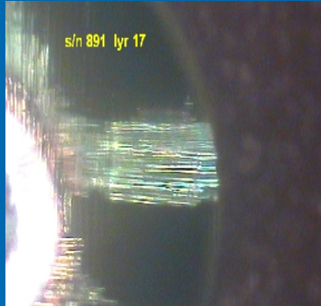
Wicking to ground
