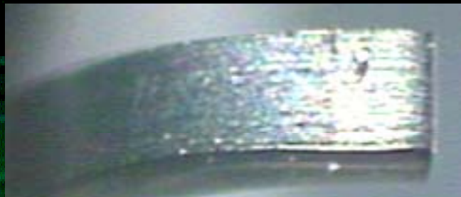
Typical lead mark with 5x hits @ 50g
