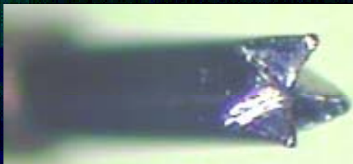
Typical lead mark with 5x hits @ 50g
